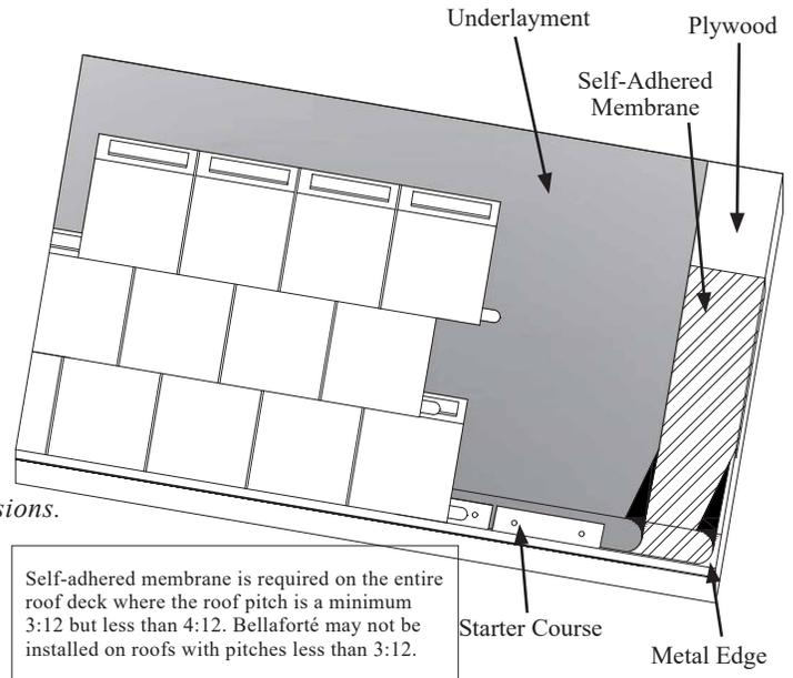
Self-adhered membrane is required on the entire roof deck where the roof pitch is a minimum 3:12 but less than 4:12. Bellaforté may not be installed on roofs with pitches less than 3:12.
