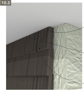
Trim screws through face of shake - Ensure the fastener penetrates the solid sheathing by at least 3/8 in.
